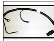
APU Harness: The old harness contained AC & DC connections as well as heater connections. The new harnesses are specific to the customer's product specifications
