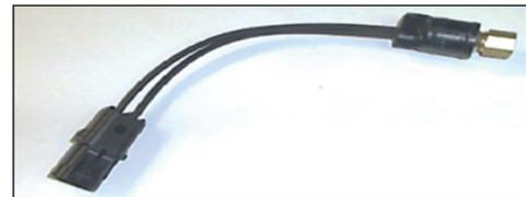
Eliminated the condenser fan relay and replaced with a pressure switch
