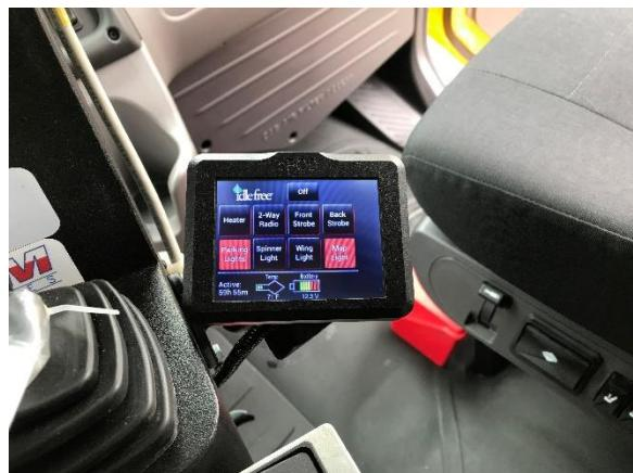
A CARB-compliant technology, Flex Systems comply with all city, municipal and state idling laws. All system functions are accessed via a small touch screen user interface located near the driver. Circuits controlled by the system are protected with a low-voltage disconnect. A timer on the touch screen displays cumulative runtime for the system making return-on-investment calculations easy for fleet managers.
